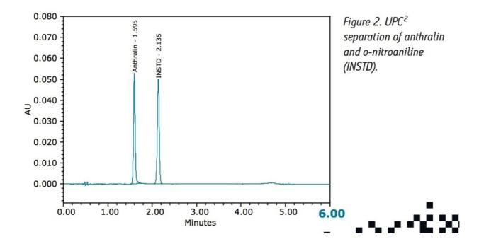
Methods converted to an SFC solution must maintain data quality (retention time reproducibility, resolution between compounds of interest and other components in the sample) and must produce results that are equivalent to the current normal phase method.
