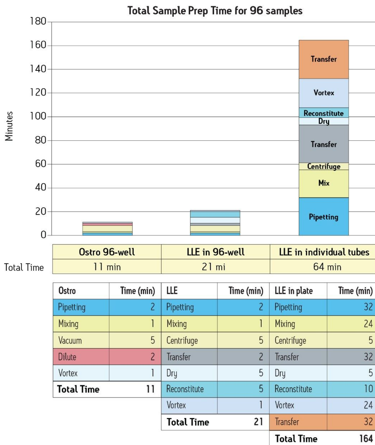
Figure 7. A comparison of the time required to prepare 96 plasma-based samples using an Ostro 96-well plate, LLE in 96-well format, and LLE in centrifuge tubes. Four LLE tubes were vortexed simultaneously. Pipetting for the 96-well plates was performed using a multi-channel pipette.
