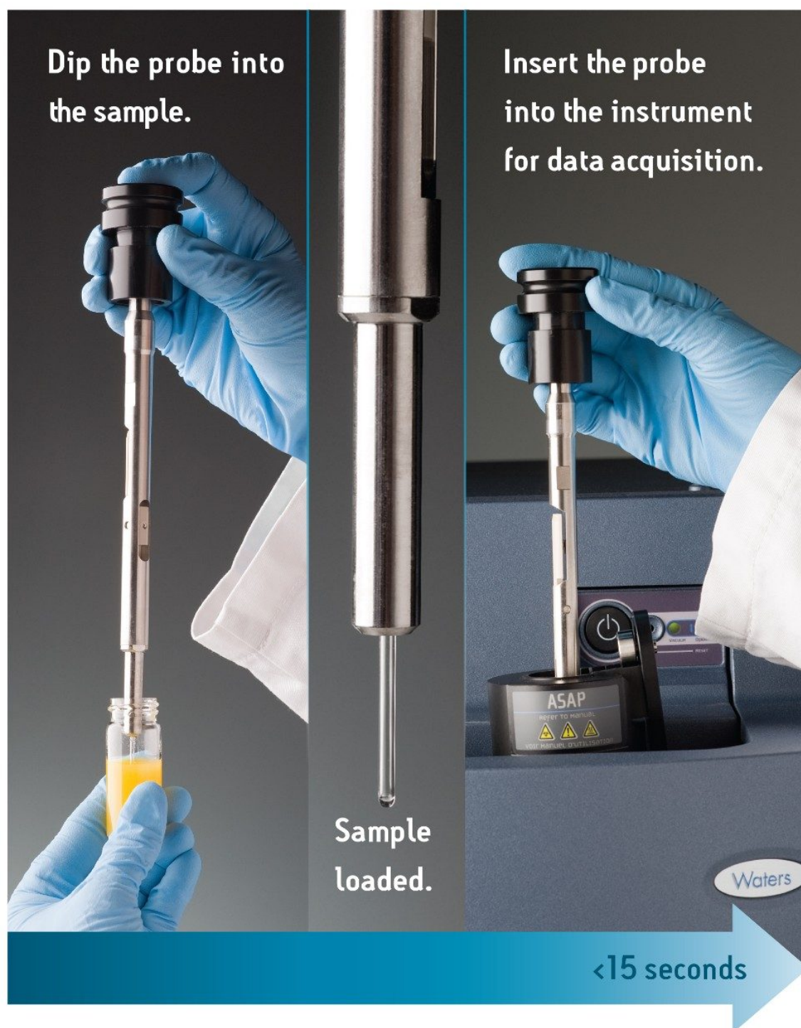
Figure 1. The sample is loaded directly onto the tip of a glass capillary. The sample is then directly inserted into
