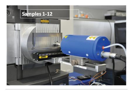
*Figure 5. Dart SVP source for Xevo instruments shown with the 12 DIP-it sampler.*
