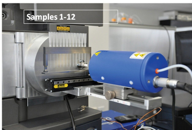
Figure 5. Dart SVP source for Xevo instruments shown with the 12 DIP-it sampler.
