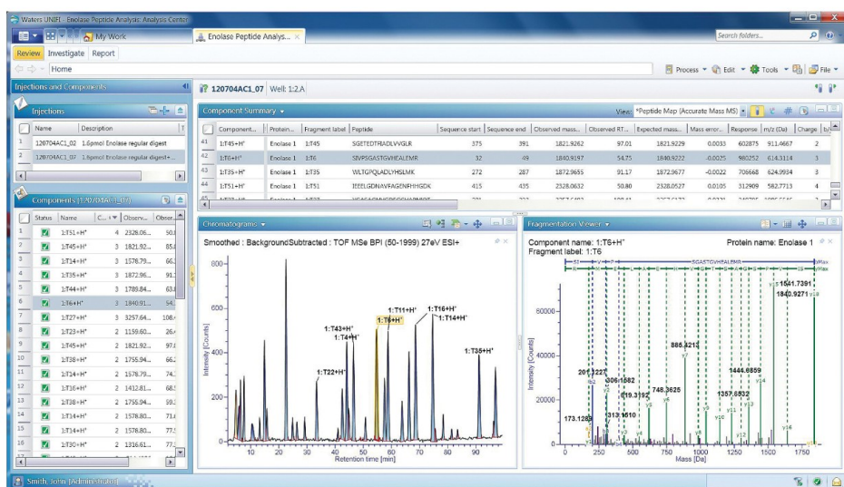
Figure 1. The Review tab in UNIFI facilitates component-driven examination of processed results for UPLC-MS E peptide mapping data.
