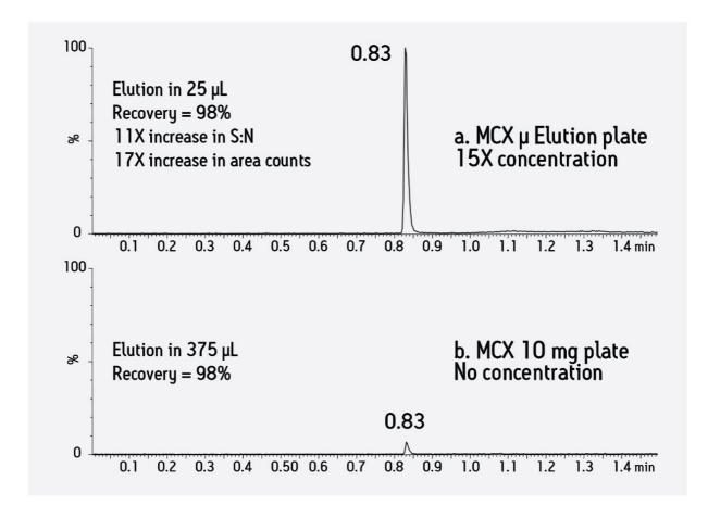
375 μL of 0.5 ng/mL risperidone in human plasma sample extracted with Oasis MCX μElution plate a) MCX μ Elution and b) MCX 10 mg.
