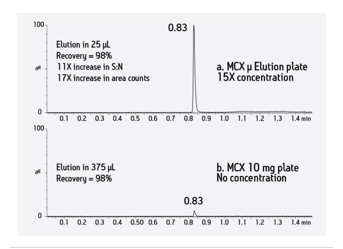
375  $\mu$ L of 0.5 ng/mL risperidone in human plasma sample extracted with Oasis MCX  $\mu$ Elution plate a) MCX  $\mu$ Elution and b) MCX 10 mg.
