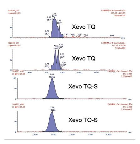
Figure 1. The same barley sample analyzed with Xevo TQ and Xevo TQ-S at a concentration of 0.1µg/kg, 20 times lower than EU legislation levels. The mycotoxin shown is Aflatoxin B1.
