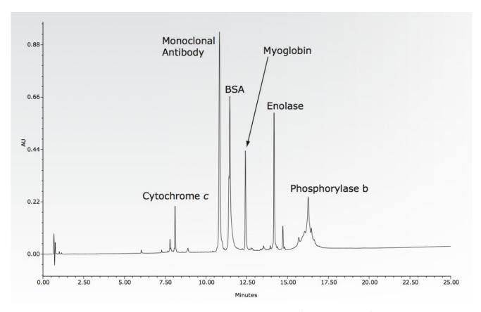
The Auto•Blend Technology method blends the required mobile phase from reservoirs of pure solvents and concentrated modifier stocks. The reversed phase chromatogram generated from this convenient method shows a wide range of proteins as a test of robustness.
