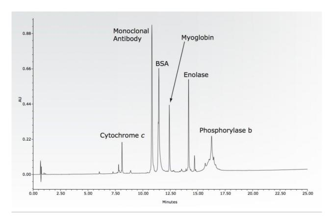
The Auto-Blend Technology method blends the required mobile phase from reservoirs of pure solvents and concentrated modifier stocks. The reversed phase chromatogram generated from this convenient method shows a wide range of proteins as a test of robustness.
