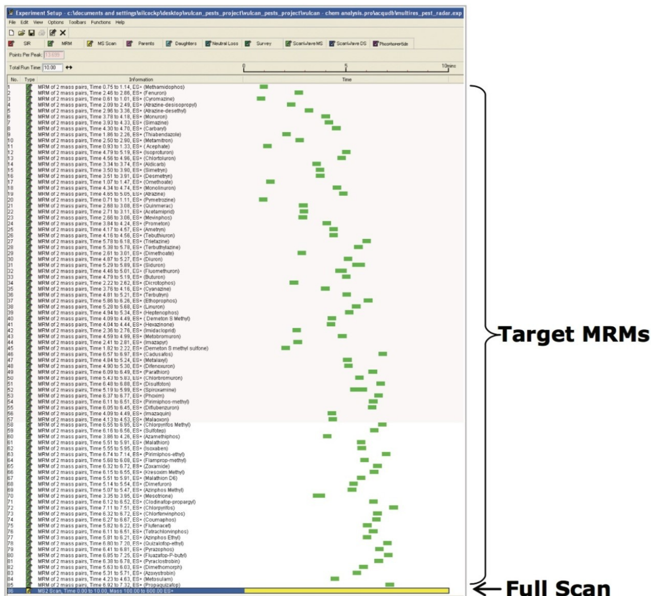
Figure 1. Mass spectrometer experiment showing RADAR acquisition mode.
