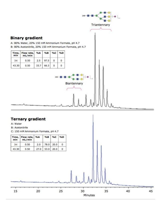
2-AB labeled glycans released from fetuin were separated using a standard binary HILIC method. The same separation was obtained in a ternary, Auto•Blend Plus mode where mobile phase preparation is easier and
