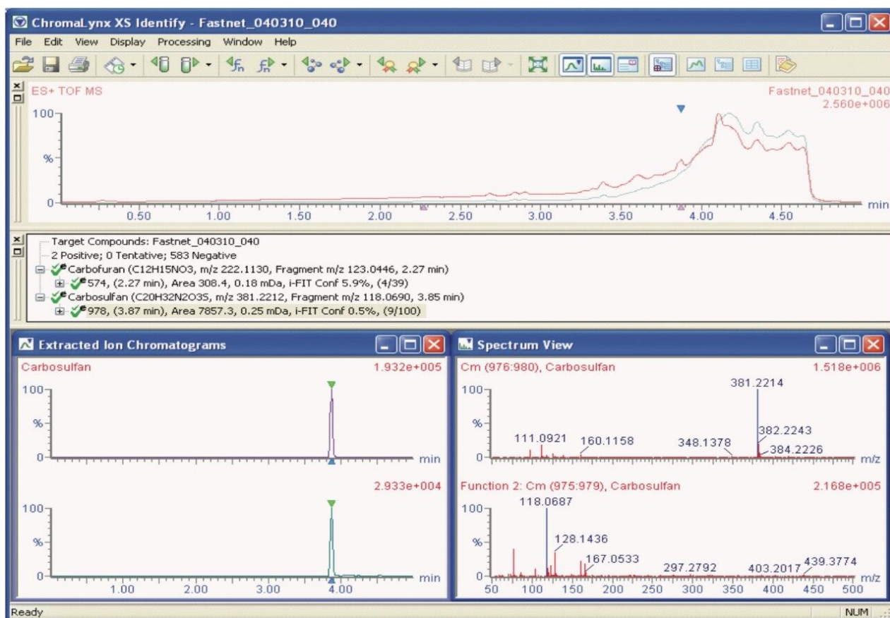
Figure 3. ChromaLynx XS Identify results browser showing MS^E precursor and fragment ion data identifying carbofuran and carbosulfan as the potential pesticide poisons.
