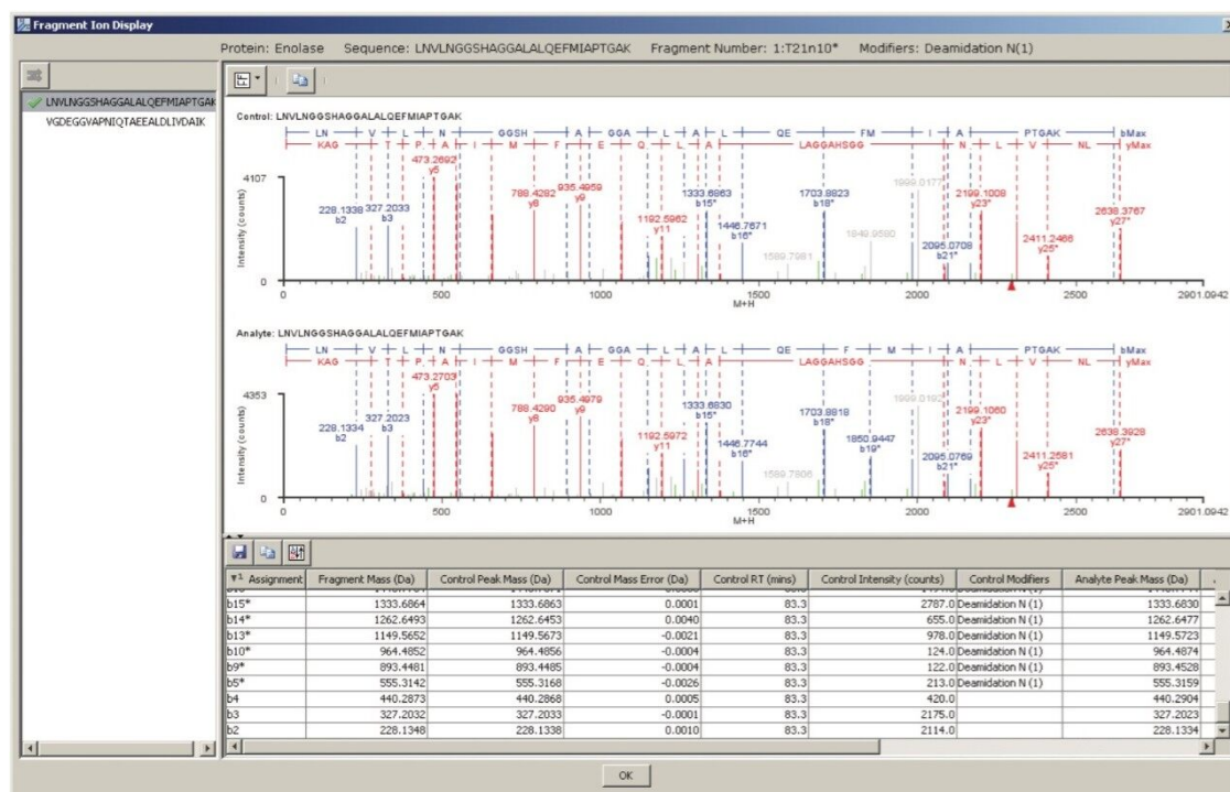
Figure 7. The Fragment Ion display from BiopharmaLynx 1.2 showing sequenced peptides on an MS/MS spectrum for a control (top) and an analyte (bottom). Additional information is available in the tabular display showing modifications and locations of these modifications.
