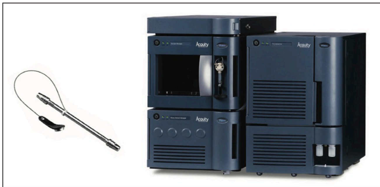
Figure 1. The Waters ACQUITY TQD system and ACQUITY UPLC column featuring eCord technology. The eCord electronically stores all the information for full traceability of your experiments including; date of column installation, certificate of analysis, number of injections, maximum temperature and pressure - a full column history.
