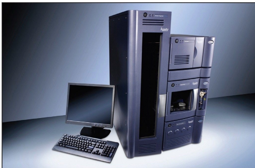
Figure 1. ACQUITY TQD with the TQ Detector.
