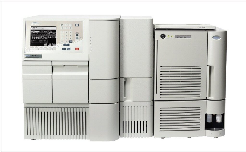
Figure 1. Alliance HPLC System comprised of the e2695 XC Separations Module and the 3100 Mass Detector.
