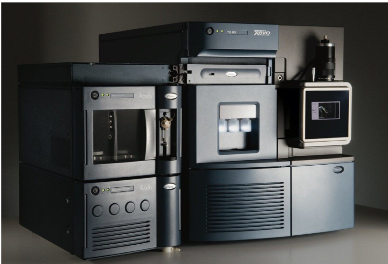
Figure 1. Xevo TQ Mass Spectrometer with the ACQUITY UPLC System.
