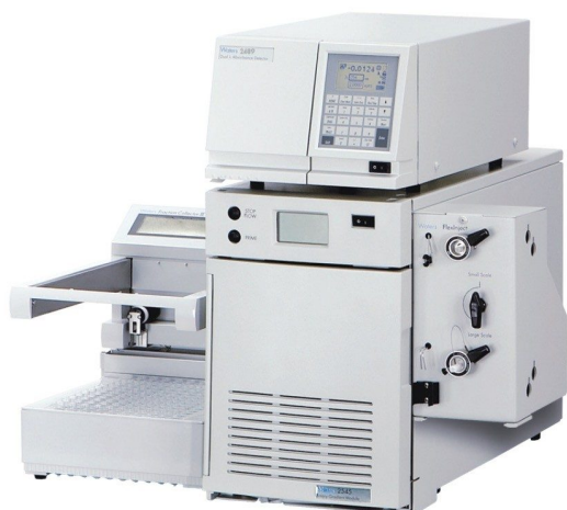
Figure 2. The Waters UV-directed purification system
