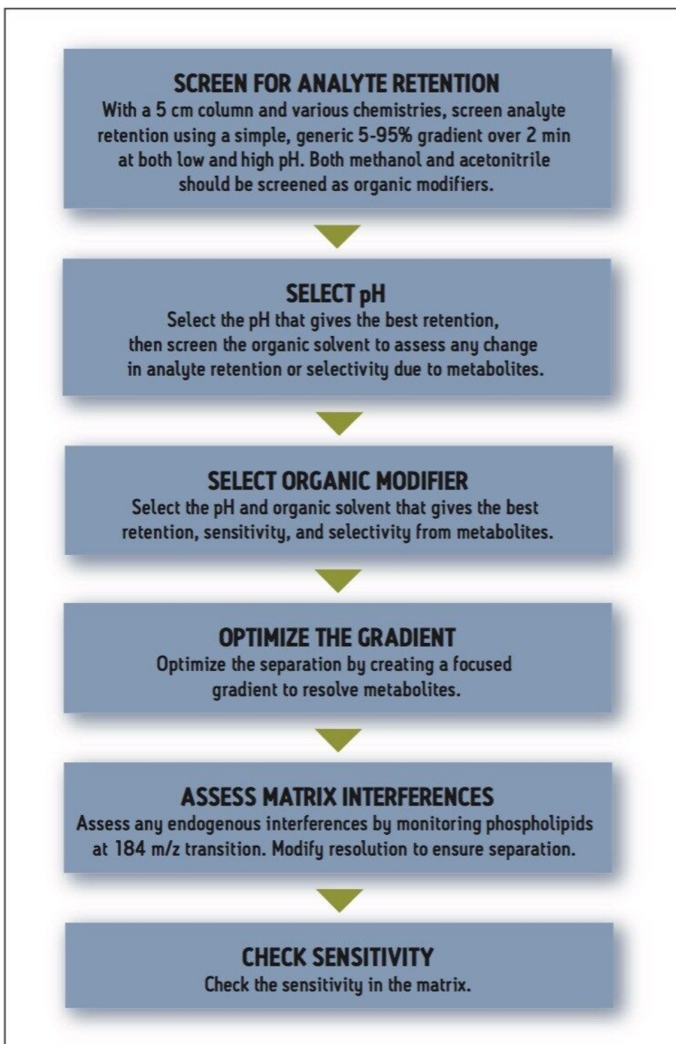
Figure 2. The bioanalytical LC method development process.
