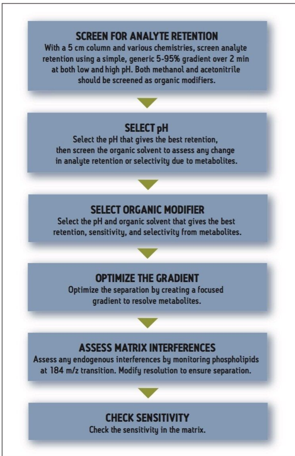
Figure 2. The bioanalytical LC method development process.
