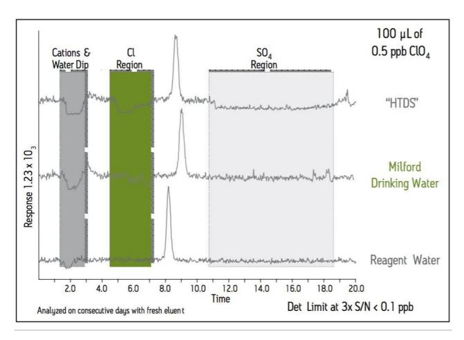
0.5 ppb perchlorate detection in three different sample matrices by LC-MS/MS.
