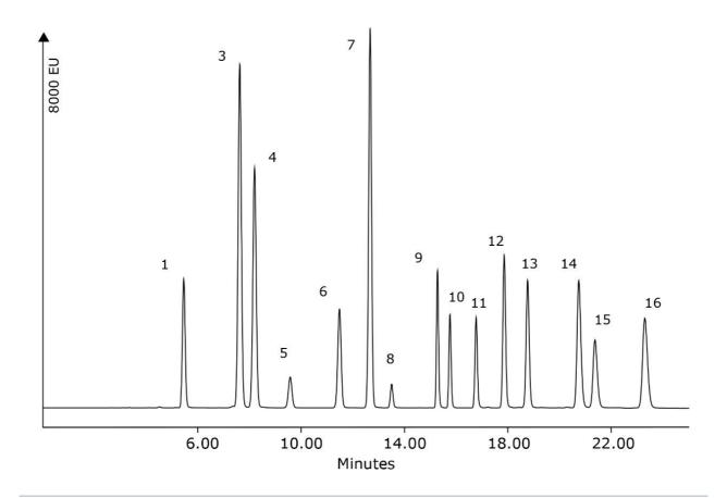
Standard chromatogram, fluorescence/programmed wavelengths, 1-20 ppm PAH analytes.
