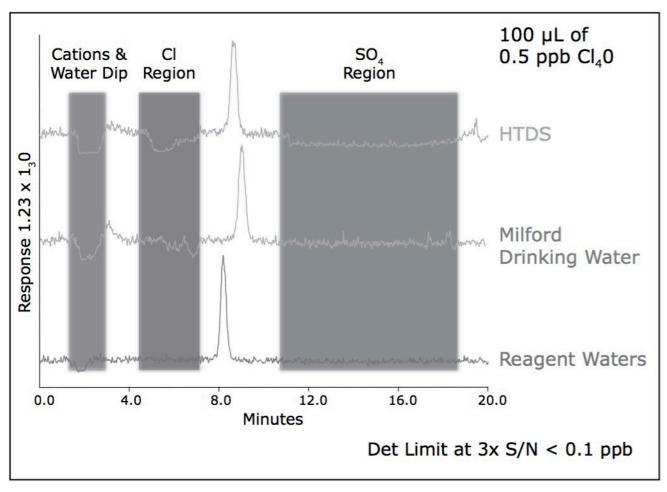
0.5 ppb perchlorate detection in three different sample matrices by LC-MS/MS. Analyzed on consecutive days with fresh eluent.
