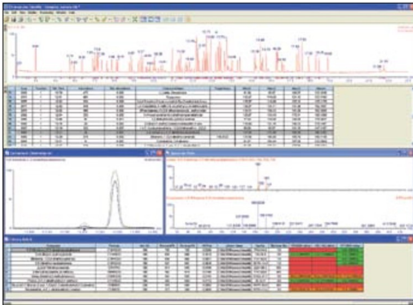
Figure 2. ChromaLynx XS Identify interactive browser report of the processed GC-MS complex chromatogram from Figure 1.
