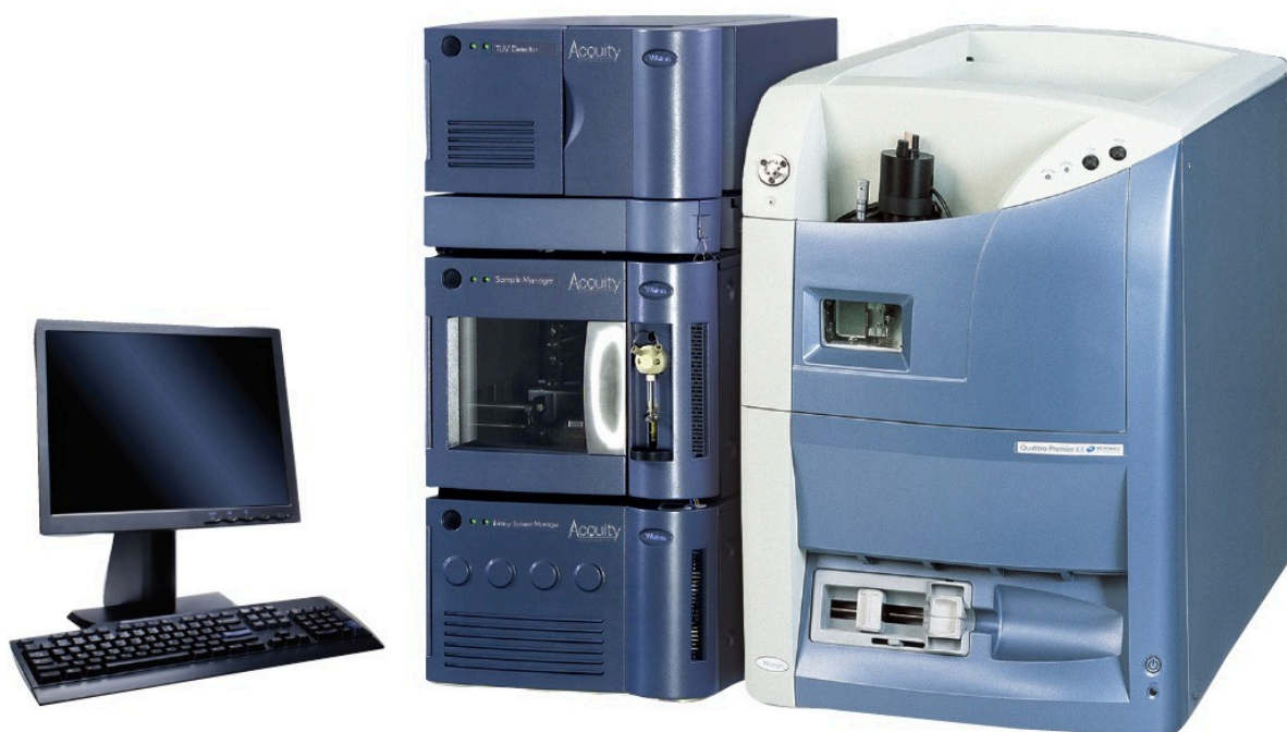
Figure 1. System configuration – ACQUITY UPLC System with a Quattro Premier XE Mass Spectrometer.
