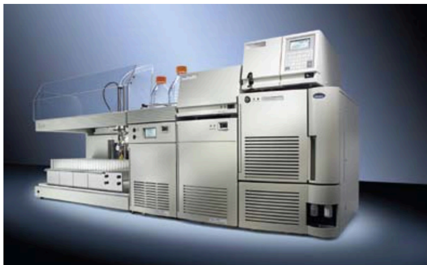
Figure 1. The mass-directed AutoPurification System consists of the 2545 Solvent Manager, 2767 Sample Manager, System Fluidics Organizer, and PDA Detector.
