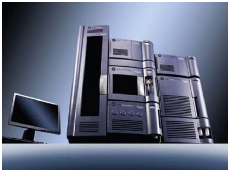
Figure 1. The ACQUITY SQD for synthetic reaction monitoring.
