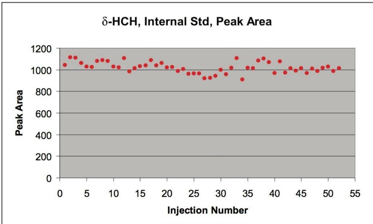
Figure 5. δ-HCH response maintained over 52 matrix injections.
