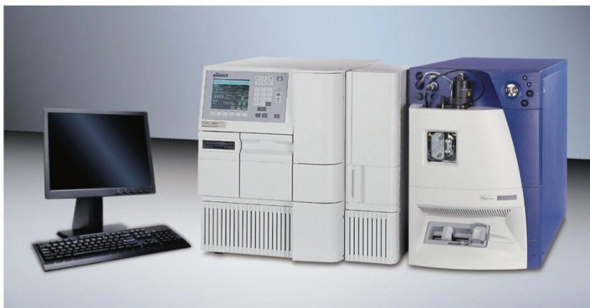
Alliance 2690 HPLC and Micromass Quattro micro mass spectrometer.
