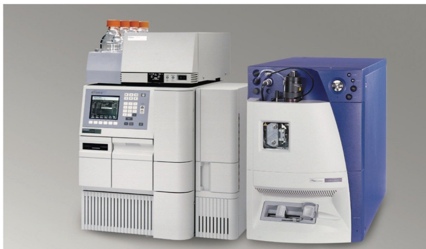
Figure 1. The Alliance HT System with the Quattro micro Mass Spectrometer.
