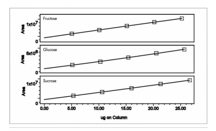
Figure 2. Calibration curves for fructose, glucose, and sucrose.
