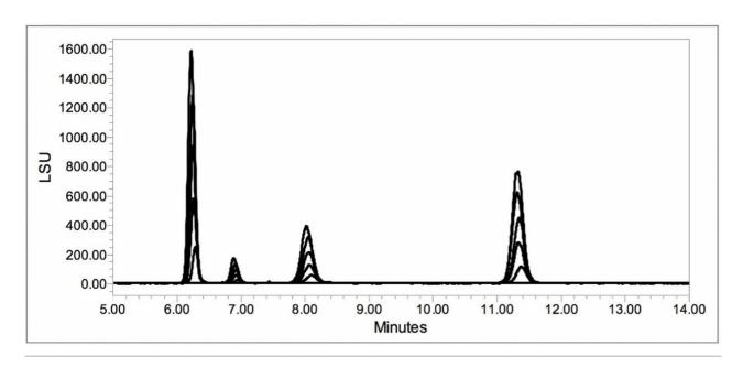
Figure 3. Overlay of fructose, sorbitol, glucose, and sucrose standards.
