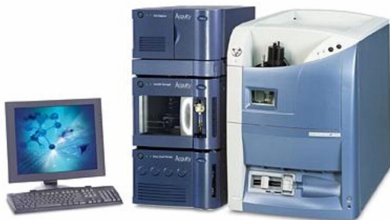
Waters ACQUITY UPLC System with the Waters Quattro Premier XE Mass Spectrometer.
