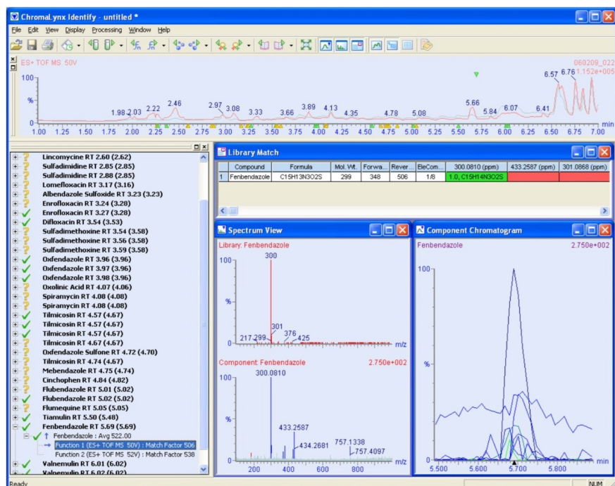
Figure 4. ChromaLynx Application Manager showing Fenbendazole successfully screened from a multi-analyte spiked milk sample at its MRL concentration (10ppb).
