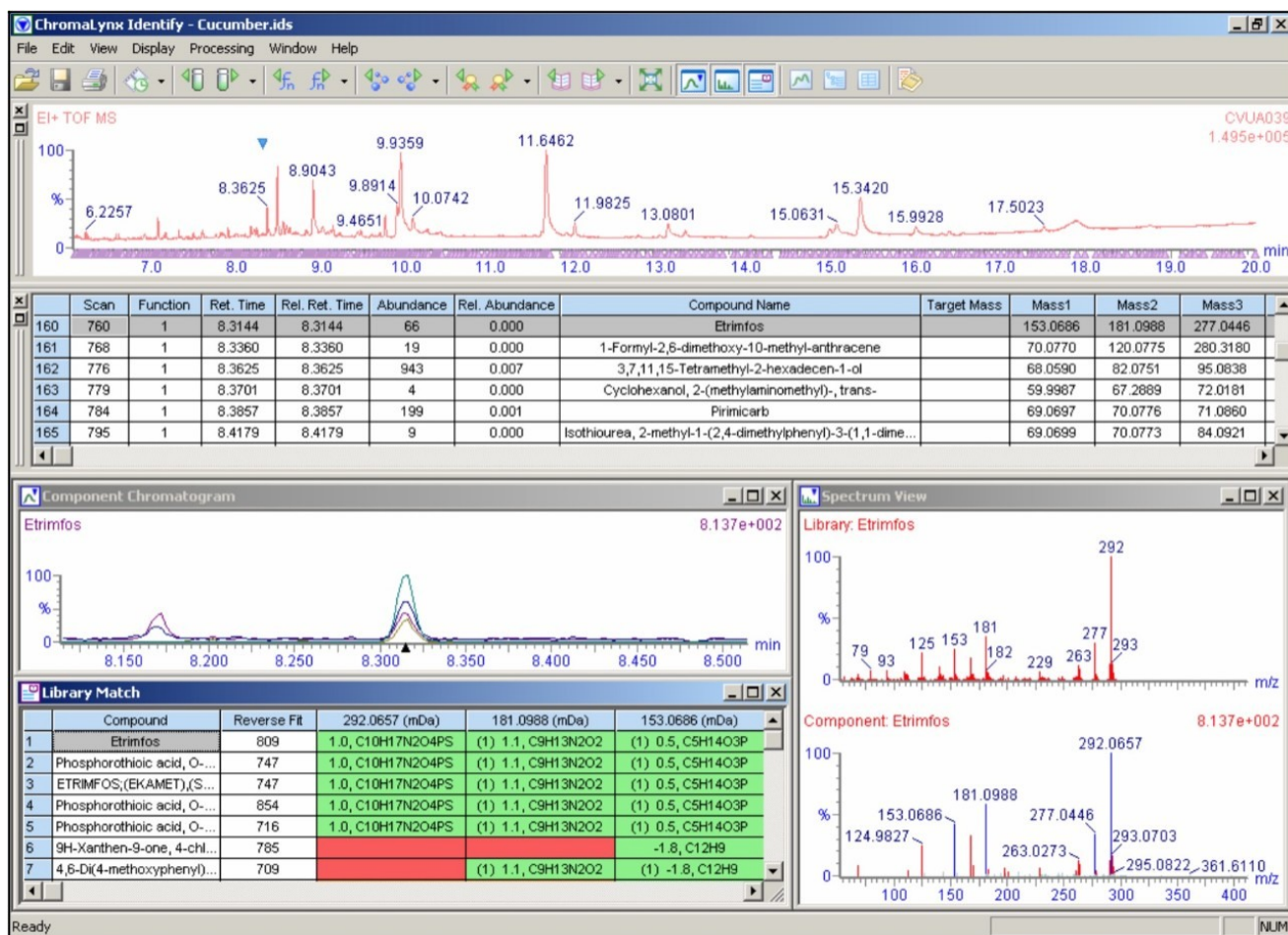
Figure 7. Example of ChromaLynx browser for an untargeted pesticide residue in spiked cucumber (0.05 mg/kg). ChromaLynx automatically performs exact mass confirmation of the library search. The formula from the library hit is submitted to elemental composition and the "n" most intense ions are confirmed/rejected by exact mass. Green boxes indicate a good exact mass match, amber boxes indicate a tentative exact mass match and red boxes indicate no match.
