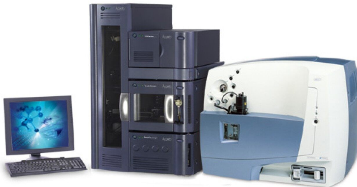
Waters ACQUITY UPLC System with the Waters Micromass LCT Premier Mass Spectrometer.
