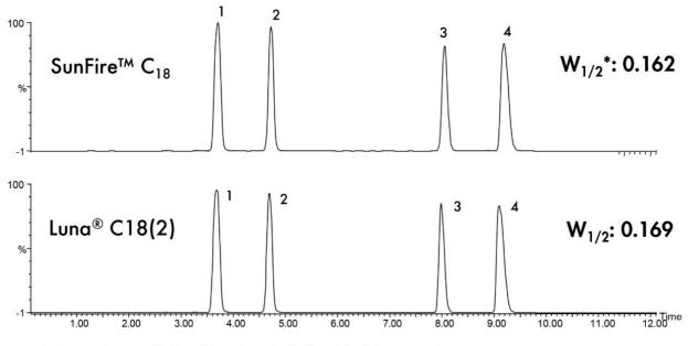
\*:  $W_{1/2}$  value is calculated based on the half width of the  $1\,{}^{s}$  peak.
