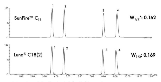
\*:  $W_{1/2}$  value is calculated based on the half width of the 1st peak.
