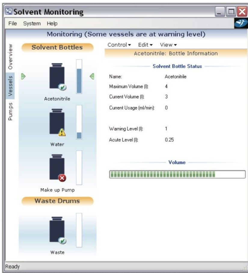
Figure 1. Each solvent container is identified. Initial and acute warning levels are entered in the vessel status page. The current volume of solvent in the 4L acetonitrile container is 3L, with an initial warning level of 1L and an acute level of 0.25L.
