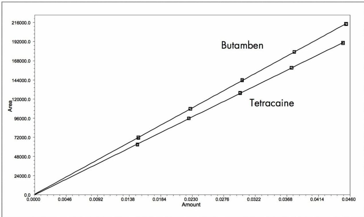
Figure 4. Calibration curves for butamben and tetracaine.
