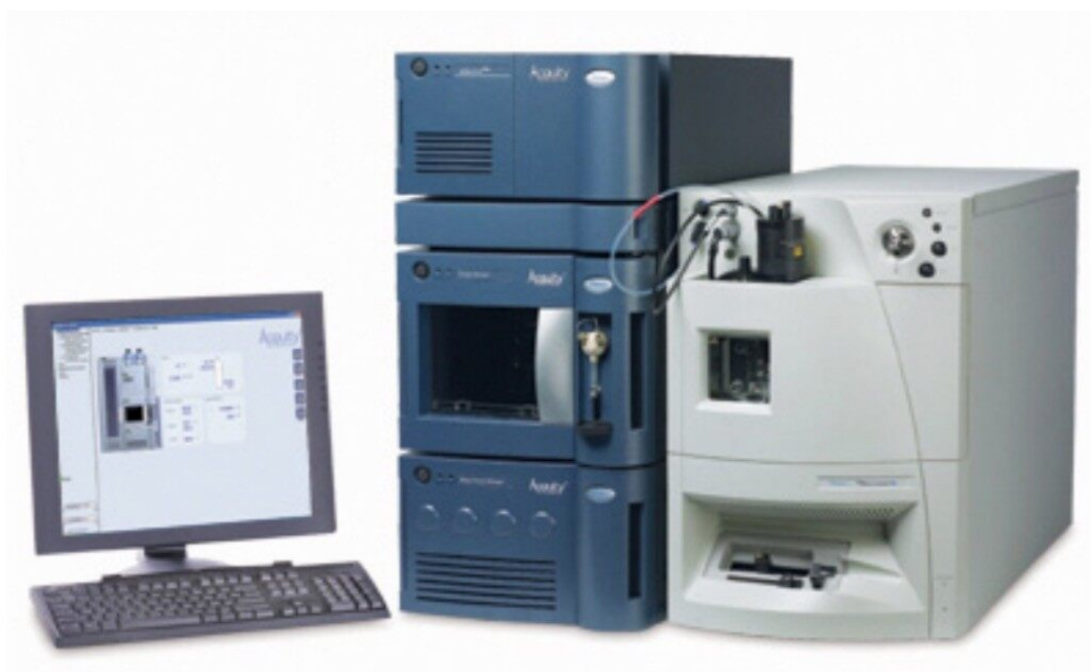
Waters ACQUITY UPLC System with the Waters ZQ 2000 Mass Detector and the Waters ACQUITY UPLC Photodiode Array Detector.
