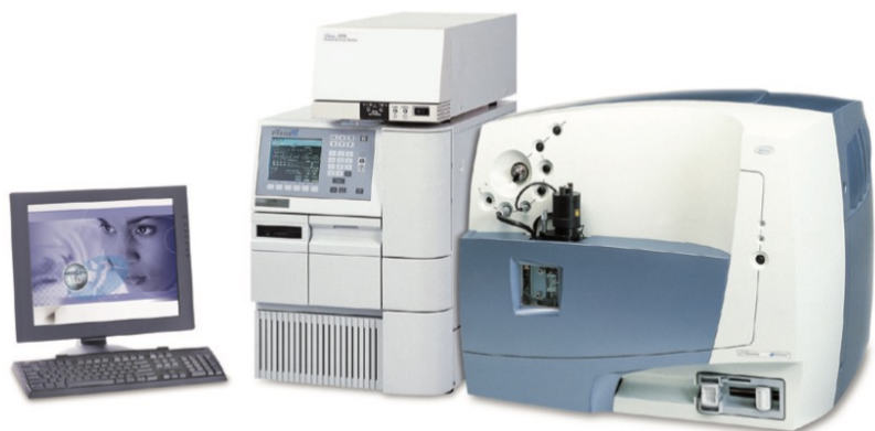
Figure 1. Alliance 2795/LCT Premier System featuring integral LockSpray.
