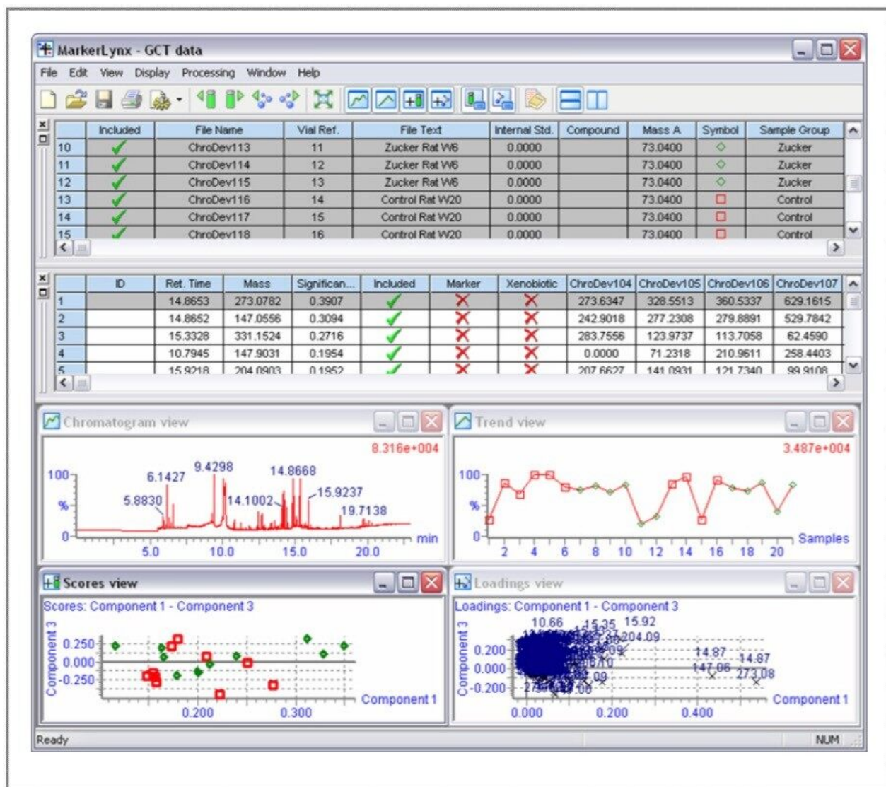
Figure 3. EI GC-MS data subjected to peak deconvolution and integration followed by PCA using the MarkerLynx Application Manager for MassLynx Software.
