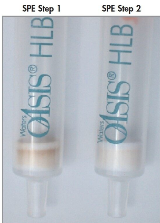
Figure 3. Left Side Column (SPE Step 1): The column on the left shows the retained matrix resulting from the initial sample pass-through. This column is discarded and the passed-through sample is then derivatized. Right Side Column (SPE Step 2): The column on the right shows the sample clean-up after the final analyte elution.
