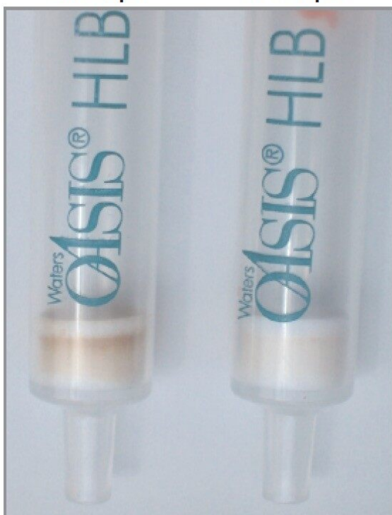
Figure 3. Left Side Column (SPE Step 1): The column on the left shows the retained matrix resulting from the initial sample pass-through. This column is discarded and the passed-through sample is then derivatized. Right Side Column (SPE Step 2): The column on the right shows the sample clean-up after the final analyte elution.
