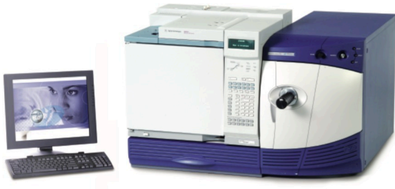
Figure 2. Waters Micromass Quattro micro GC MS System.
