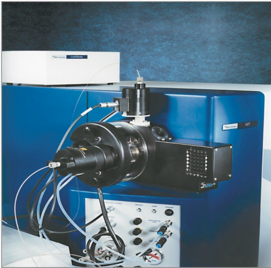
Figure 1. Dual electrospray source mounted on an LCT oa-ToF instrument.
