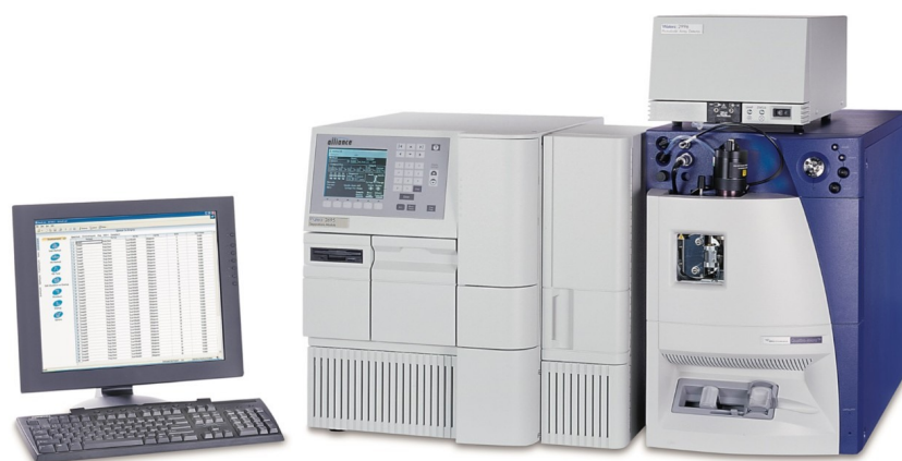
Waters Micromass Quattro micro API Mass Spectrometer, together with Waters Alliance 2695 Separations Module, 2996 PDA Detector and MassLynx Software.
