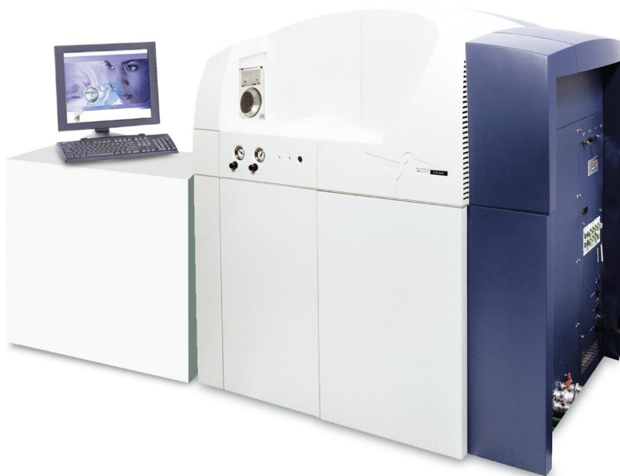
Waters Micromass Q-ToF Ultima MALDI Mass Spectrometer.
